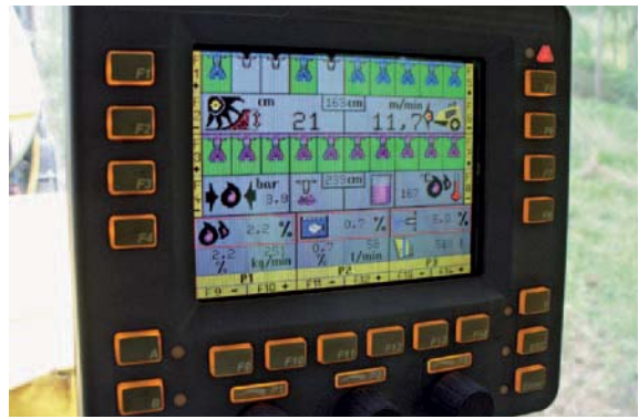
Process control by dosing computer.
